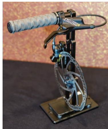
▲ Tektro's HD-M745 entry-level, quad-piston disc brake.
