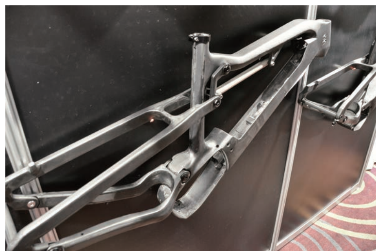
▲ The downtube is designed for battery integration, to give the frames greater aesthetic appeal.
