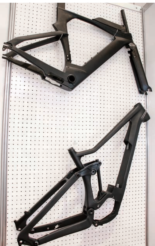
▲ The upper frame is for a TT bike, and the lower for eMTBs.
