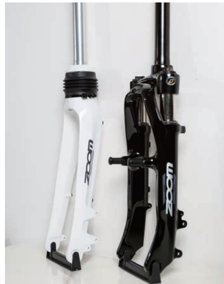
▲ Zoom's 106 single-crown fork (left) is suitable for centrally-mounted and rear-wheel drive electric motors; the 730 double-crown fork (right) is suitable for front-wheel drive e-bikes.
