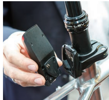
▲ Magnets guide Monkey Link accessories effortlessly onto the ports.
