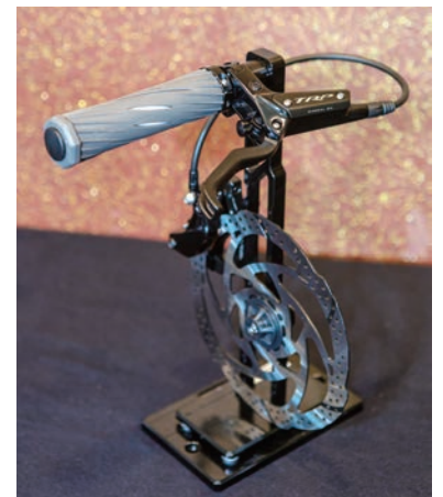
▲ Tektro / TRP's HD-E840-2 eMTB disc brake.
