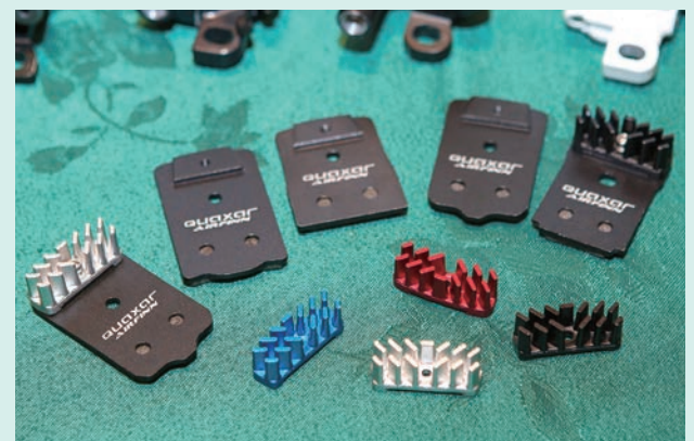
▲ Quaxar's Air Finn pads feature removable heat sinks.
